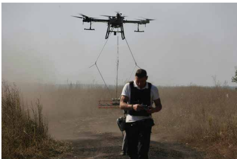
A Ukrainian researcher tests an unmanned aerial vehicle-based system to detect landmines, which is being developed with support from NATO's Science for Peace and Security Programme. Kharkiv, Ukraine, June 2023. Photo credit: Vyacheslav Madiyevskyy.
