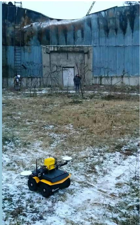
Preliminary test for the navigation of one of the Demining Robots platforms. Kharkiv, Ukraine, January 2023.
