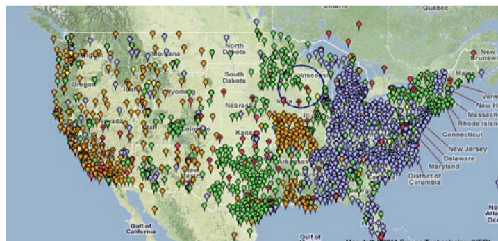
Figure 3. U.S. CORS Station Locations
