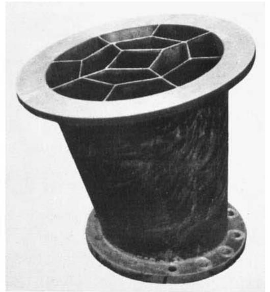
Fig. 13. The "Honeycomb" Diffuser used in the First Model of the Experimental Engine
