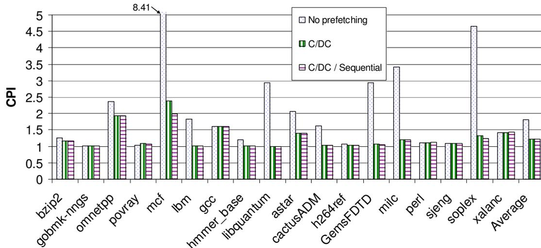
Figure 11: CPI for C/DC based prefetching schemes over all simulated benchmarks.
