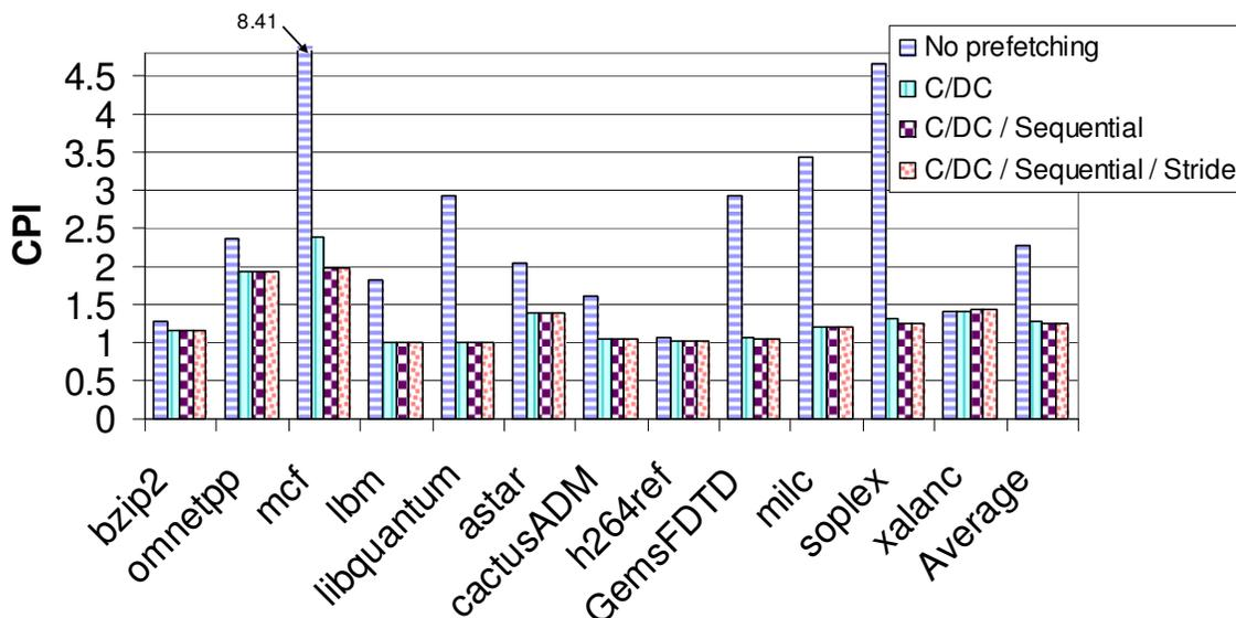
Figure 4: CPI for C/DC and C/DC Hybrid prefetching schemes.
