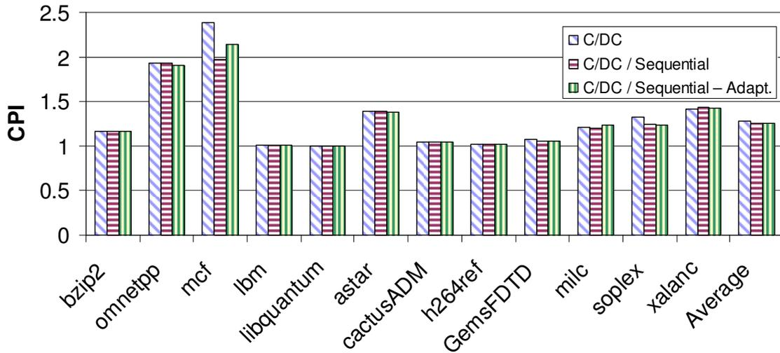
Figure 7: CPI for C/DC based Hybrid Adaptive Schemes.
