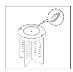
Please ensure the bottom screw is tightened before installation.
