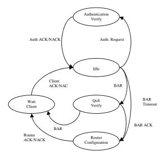
Figure 7 - Negotiation Protocol in the Server: State Diagram
