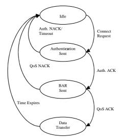
Figure 5 - Negotiation Protocol in the Client: State Diagram
