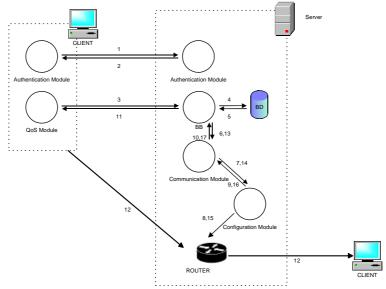
Figure 9 - Functional modules of the prototype
