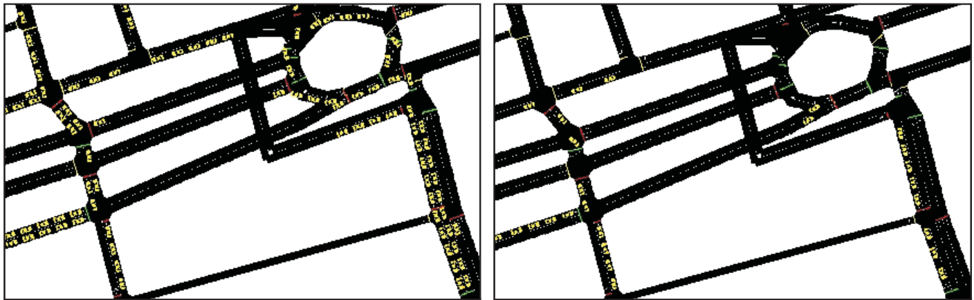
Fig. 11. Simulation traces of the traffic flow (cars in white) resulting from the cycle programs generated by both, SCPG (left) and PSO (right). The pictures show snapshots at the end of the simulation time. The reader can see that the SCPG leaves a dense traffic while PSO has cleared the routes and the traffic is very fluid and smooth
