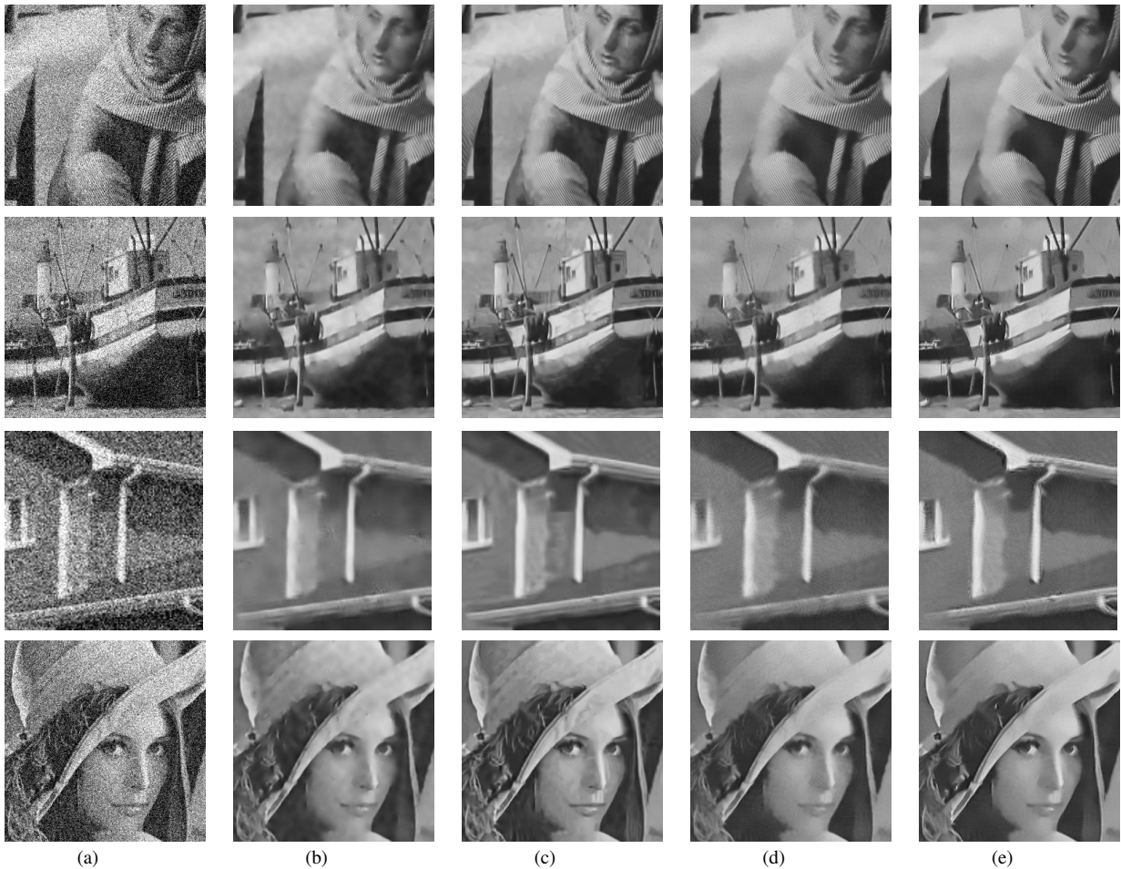
Fig. 3. (a) From top to bottom, corrupted images of Barbara , Boat , House and Lena by an additive WGN with standard deviation \sigma = 40 . Denoised images using (b) the K-SVD filter, (c) the BM3D filter, (d) our non-iterative PPB filter (i.e the NL-Means filter) and (e) 25 iterations of our PPB filter.
