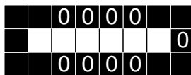
Figure 5: We can fix terminate both ends of this wire to form a complete Boolean circuit. The 0 on the right forces us to place a light bulb at the beginning of the wire on the left; we have found a satisfying truth assignment for this circuit.
