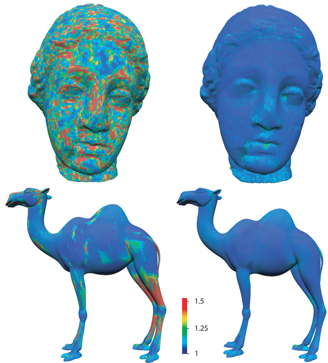
Figure 10: Two examples ( Hygeia , genus zero; cut camel with free boundaries) comparing distortion for original triangulation (left column) and iDT (right column). (Used with permission from [Kharevych et al. 2006].)
