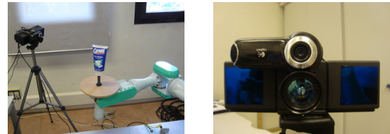
Figure 1. Left: PMD Camcube 2.0 coupled with a color camera. Right: Turn-table setup using a PA10 robot.
