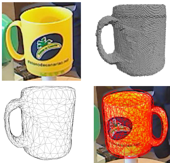
Figure 3. Example of acquired model: cup. Top left: object to scan, top right: carved volume, bottom left: Poisson reconstruction, bottom right: reprojection on a color image with known pose.
