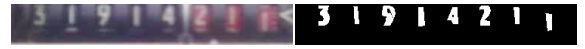
Figure 5. Input/output training example for the digit segmentation problem. The figure-ground segmentation map has been segmented by hand to train the model to recognize and segment only the digits of the meter.
