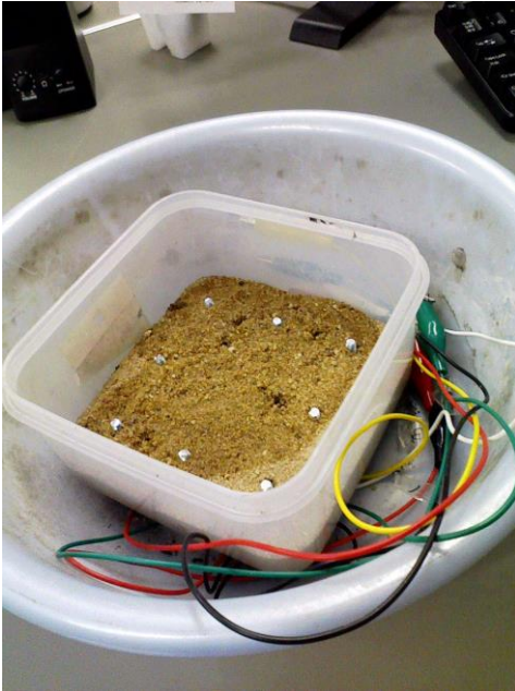
Fig.5 Small size 2D sand box model and water injection device (syringe).
