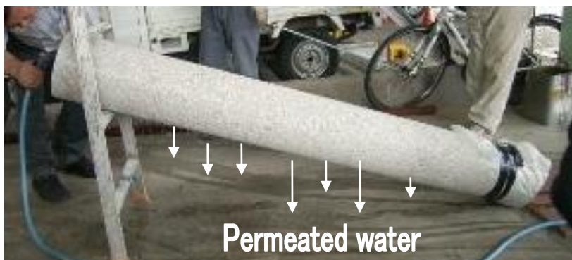
Fig.1 Water permeable pipe. \phi :0.2-2m, Length: 2-6m.
