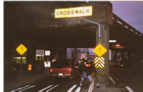
Figure 70: An overhead crosswalk sign used in conjunction with double bar pair crosswalk markings and pedestrian crossing signs in Seattle, Washington.
