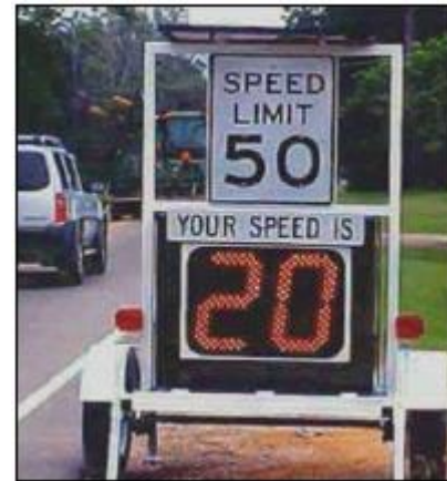
Figure 78: A portable speed trailer that displayed driver speed used in a San Francisco, California, evaluation study
