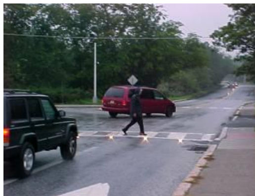
Figure 11: In-pavement flashing lights used at a crosswalk in Vermont.
