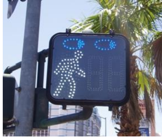
Figure 38: A pedestrian signal with animated eyes used in Las Vegas, Nevada.
