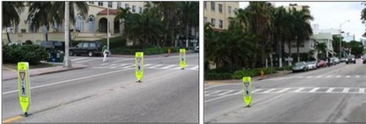
Figure 68: Two placements of in-roadway pedestrian signs as tested in a Miami, Florida evaluation study.
