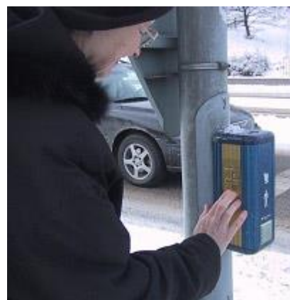
Figure 50: A pedestrian using the tactile surface of an accessible pedestrian signal
