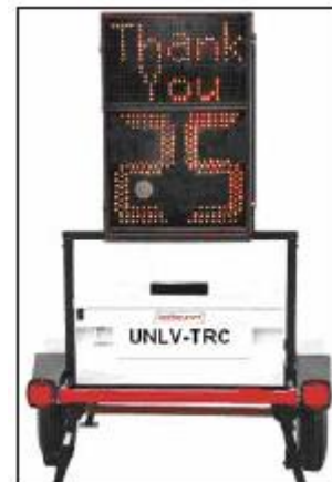
Figure 79: A portable speed trailer that displayed driver speed used in a Las Vegas, Nevada, evaluation study.
