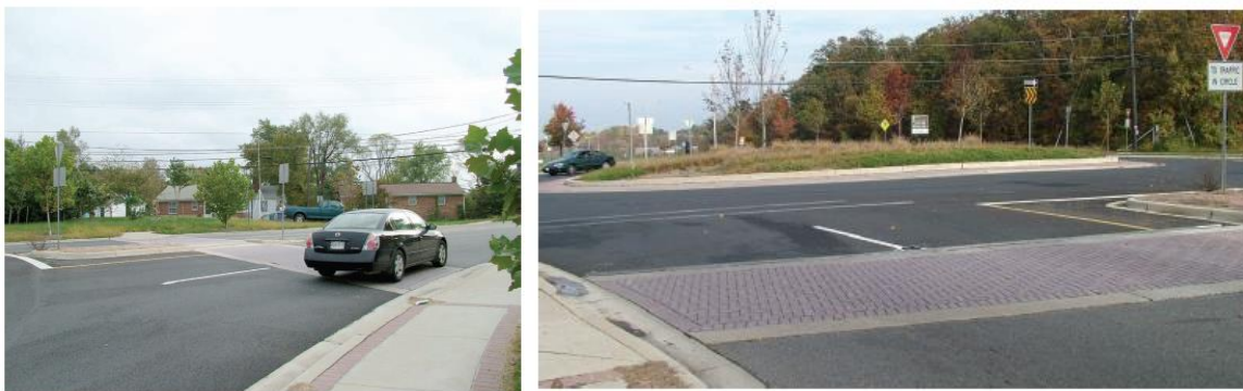
Figure 32: A roundabout treated with sound strips.
