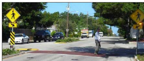
Figure 56: A pedestrian crosses in a crosswalk where pedestrian crossing signs have been enhanced with RRFBs, Miami, Florida
