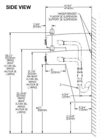
NOTE: A service supply stop must be installed at the cooler inlet tube. Adult ADA requirement. 24" (608mm) for child ADA. Adjust other measurements accordingly.
