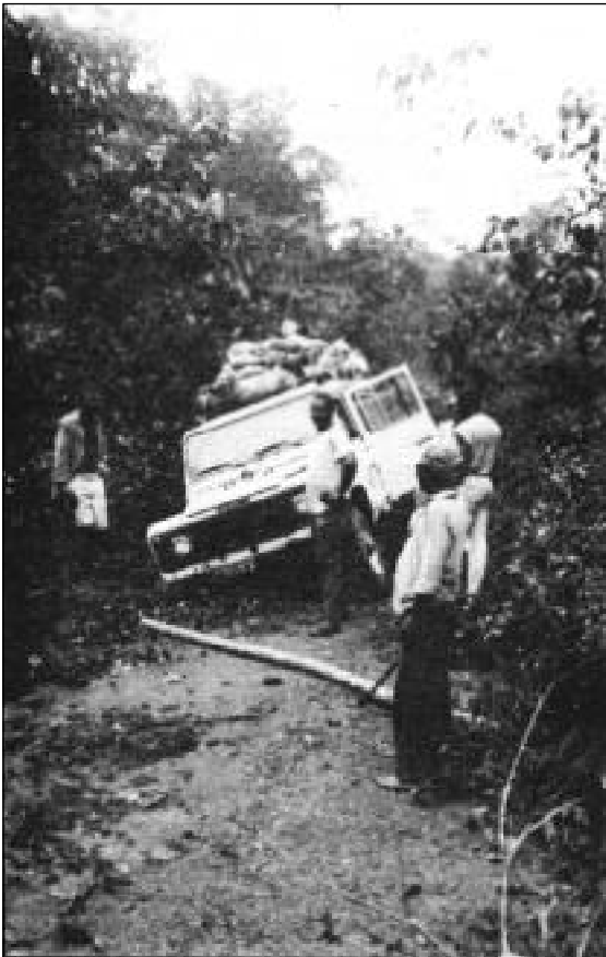
This accident, which befell us in November, 1990, illustrates the dangers of traveling on abandoned logging roads. Large tree trunks spanning a stream bed had rotted through, leaving a 'trap' concealed by vegetation. The vehicle came to rest on its axles, half suspended over a 12 foot drop to the river bed below.
