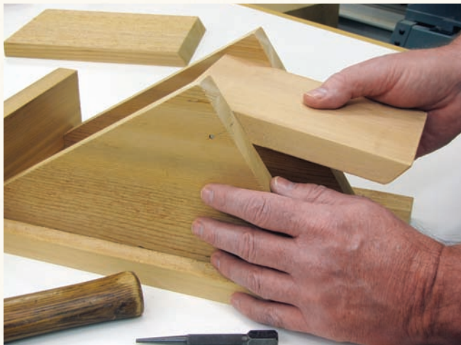
FIGURE 3 Install a galvanized nail through each side to act as hinges.
