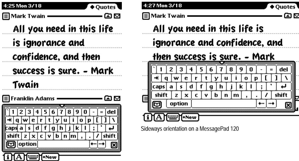
Figure 1-3 An application adjusts its size, position, and layout to fit the screen
