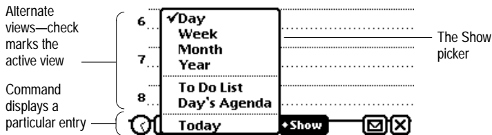
Figure 4-19 The Show picker lists alternate ways to see an application's data
