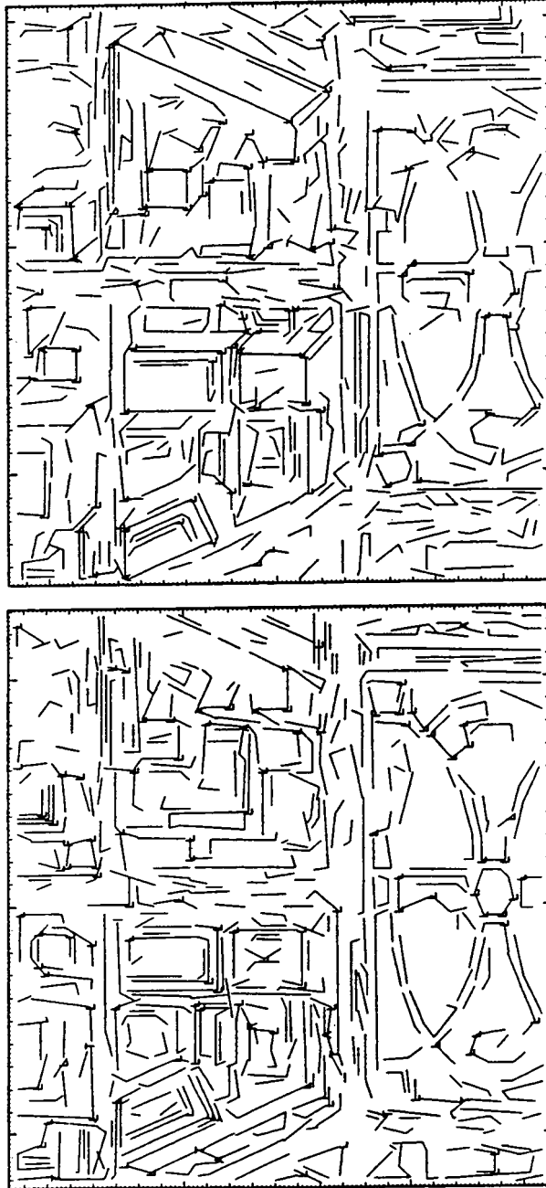
FIG. 5. Result of classifying junctions extracted from the images in Fig. 4. Junctions are classified as L, A (arrow), F (fork), or T.
