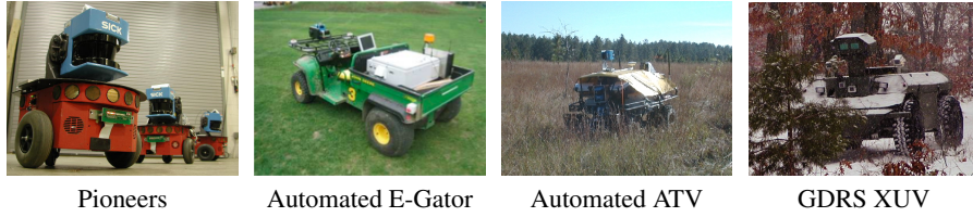
Fig. 4. Some robots that currently use Field D* for path planning. These range from indoor planar robots (the Pioneers) to outdoor robots able to operate in harsh terrain (the XUV).
