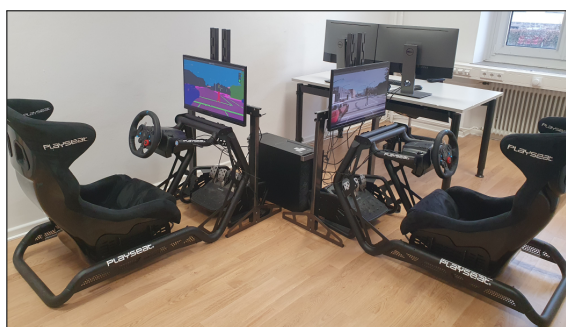
Figure 2: Test rig including steering wheels, pedals, seats and screens.
