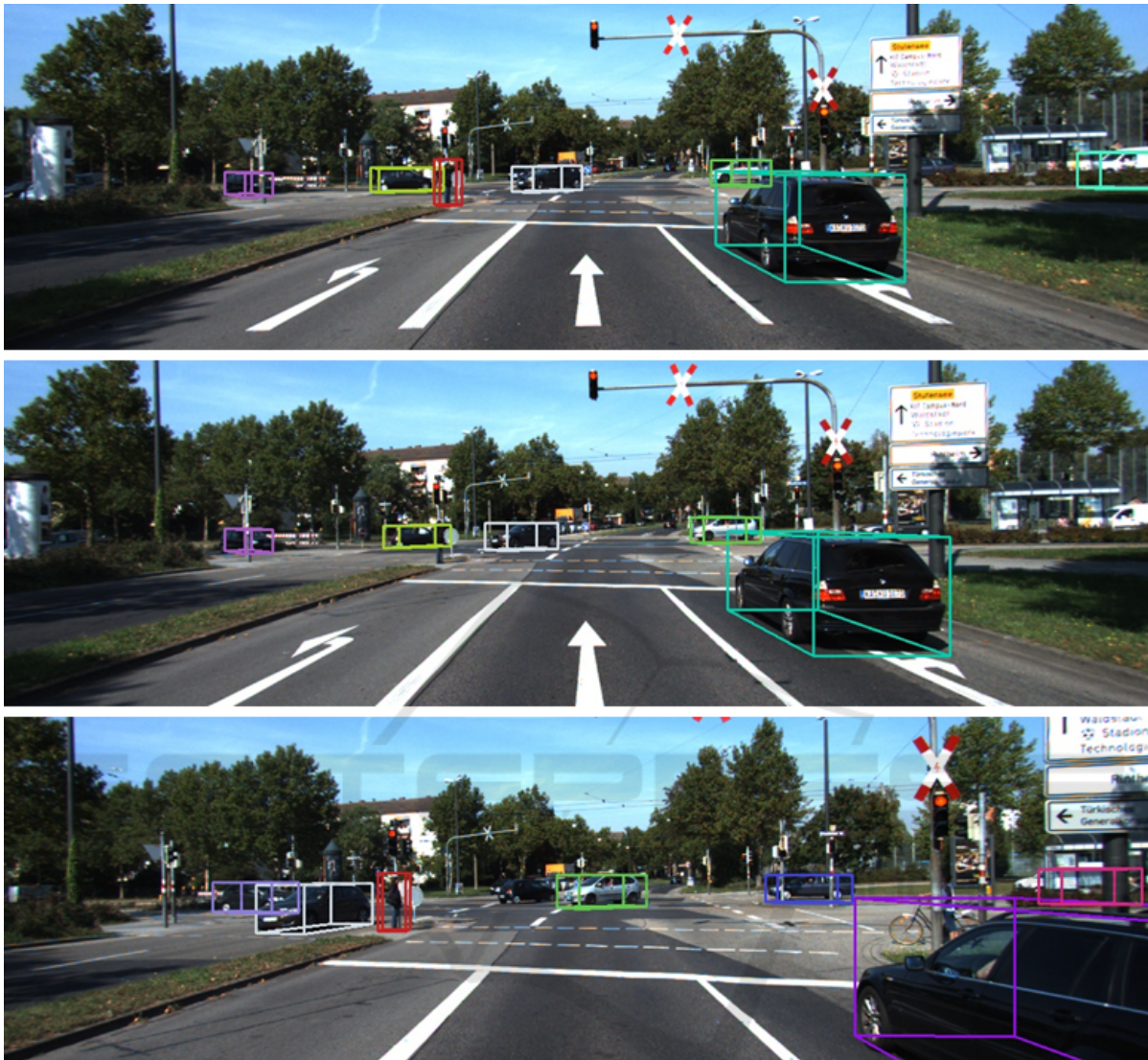
Figure 3: Qualitative tracking results of the proposed method on the KITTI validation set. Same coloured bounding boxes denote the same track identity assigned.
