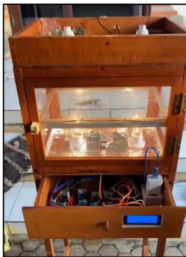
Figure 3: The shallot instore hybrid dryer model.
