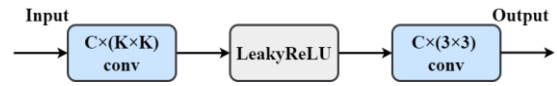
Figure 3: The size of the convolution kernel K in the Inception module is 1, 3, 5, and 7 convolution layer structures
