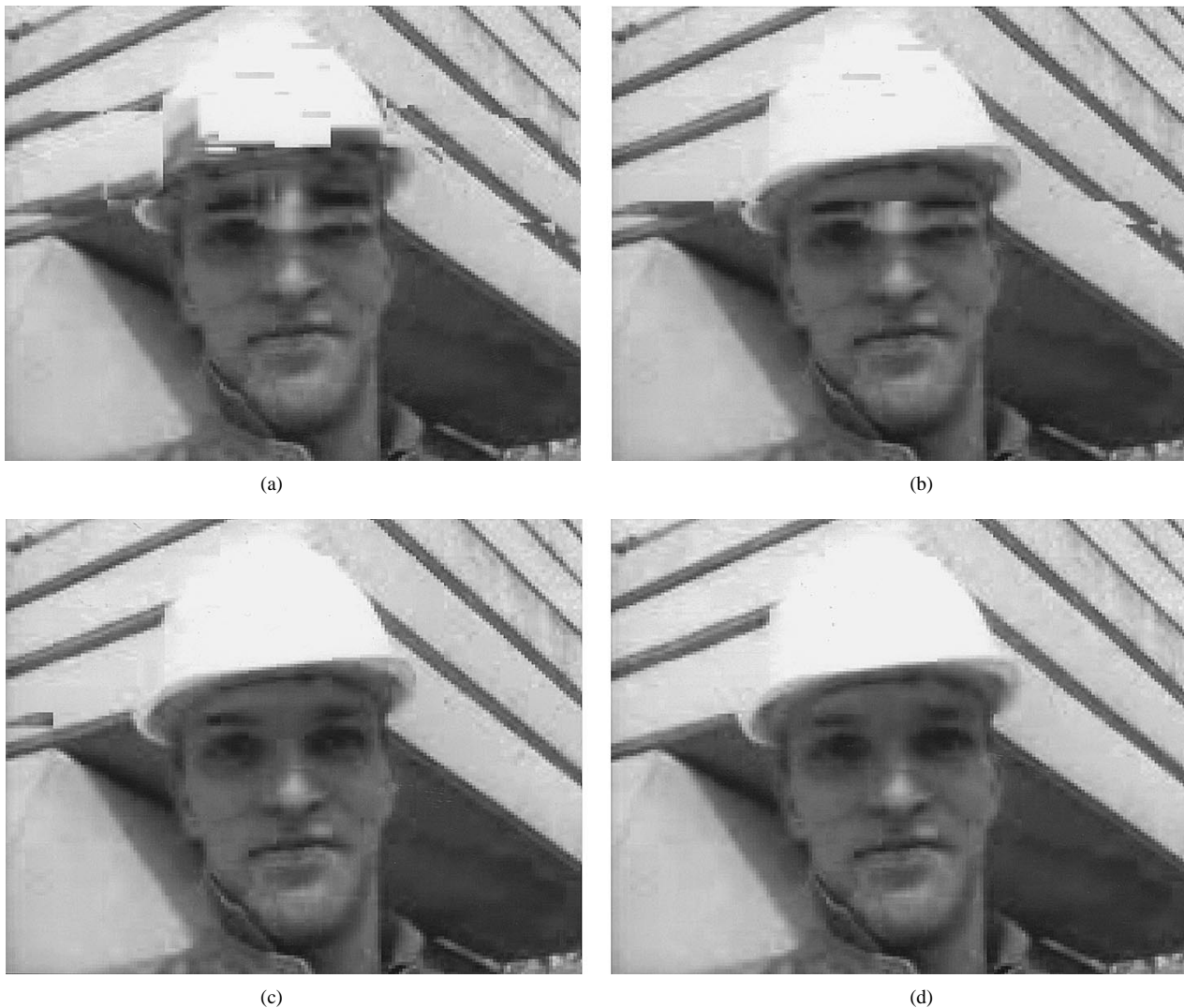
Fig. 7. Reconstructed frames of test sequence Foreman : (a) frame 90 after previous frame concealment of two GOB's in frame 75; (b) as (a) with INTRA update in frame 90 according to Same GOB strategy; (c) as (a) with INTRA update in frame 90 according to error tracking strategy; (d) frame 90 without GOB loss in frame 75.
