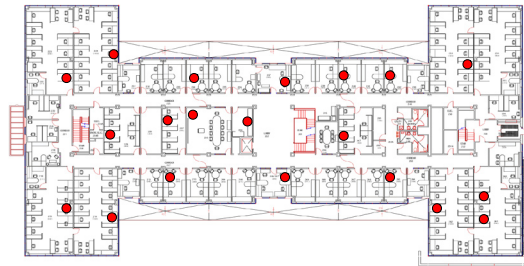
Figure 5: Experimental testbed with dots representing nodes.
