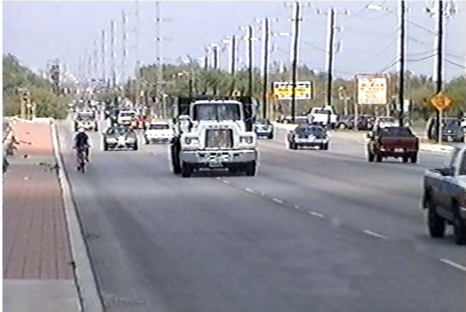
Figure 7.9. Truck passing a cyclist on a wide outside lane
