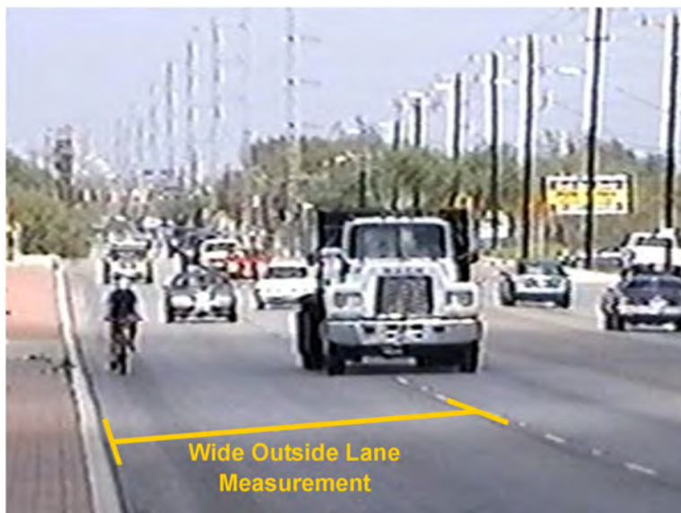
Figure 7.4. Example measurement from a roadway with a wide outside lane
