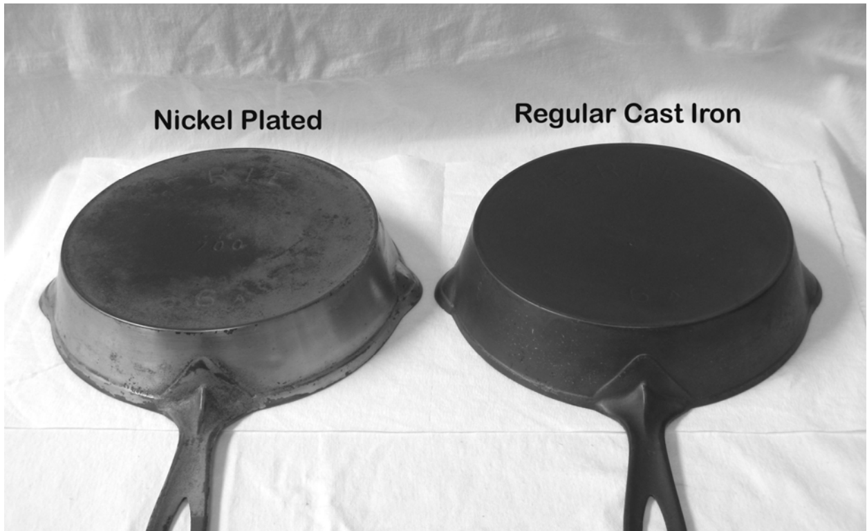
Figure 14. Comparison of nickel-plated and regular (unplated) cast iron
