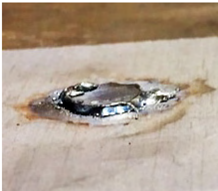
Spot weld on bottom plate
