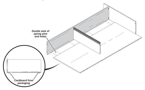
8. Place one shelf pin (32) into the side panel under the center of the fixed shelf.
