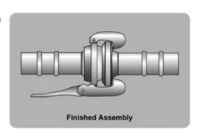
The Wil-loc B-Style Ball and Socket Coupling is a quick action coupling consisting of four components:
