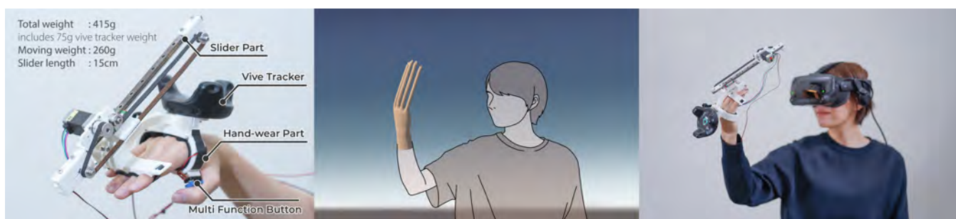
Figure 1: WeightMorphy is a hand-mounted VR controller designed to provide passive haptic feedback by changing the moment of inertia. It allows for comfortable manipulation of virtual or tele-bodies with various hand shapes.
