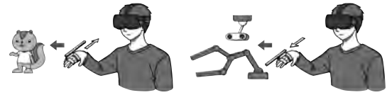
Figure 3: WeightMorphy Concept. The slider shifts backward (left) when controlling a small cartoon character-like virtual hand, and it shifts forward (right) when controlling a large robotic hand.
