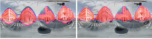
Fig. 3: Camera-pose refinement result. Compared with a registration result using a raw camera pose from Google Street View (left), building models (red) on the right-hand image are better aligned with a street-view image when using a refined camera pose computed by image-model registration deploying inferred semantic information.
