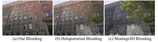
Fig. 6: Blending result comparison. Compared with our blending weight that considers the user’s current position, Holoportation [39] sets a weight using cosine between a surface normal vector and a resource-camera vector, whereas Montage4D [15] uses cosine between a user’s camera vector and a resource-camera vector. Since our method can recognize that trees behind a user are invisible in the current view, proper building-texture colors are mapped without the trees.
