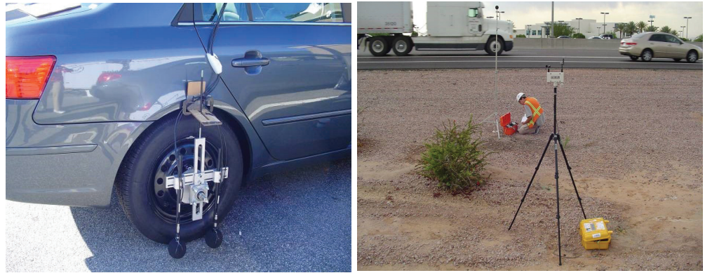
Figure 7. Left: onboard sound intensity (OBSI) measurements. From Pavement Effects Implementation Study (Rochat et al., 2012). Right: wayside noise measurements. Continuous-flow traffic time-integrated measurements from Arizona Quiet Pavement Pilot Program. Available at http://acousticstoday.org/jrochat/ .
