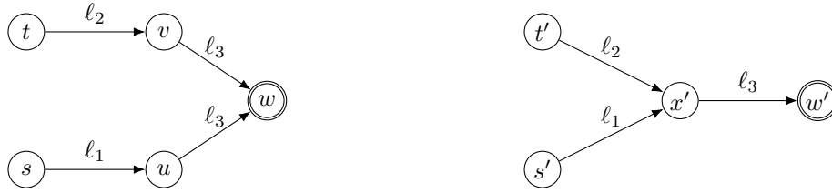
(a) Transition system \Theta with bisimilar states u and v . (b) Transition system \Theta^\alpha induced by \Theta and \alpha .
