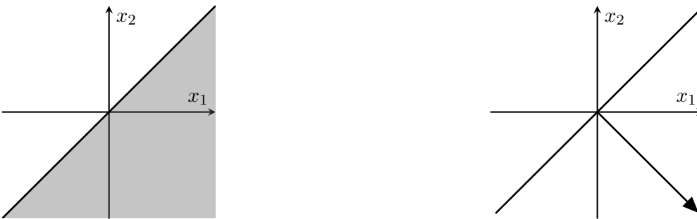
Figure 3.3: On the left hand side we have the polyhedral cone C = \{x \in \mathbb{R}^2 \mid -x_1 + x_2 \leq 0\} . The right hand side shows its decomposition into the lineality space and a pointed polyhedral cone. The lineality space is depicted by the straight line from bottom left to top right. The pointed polyhedral cone only consists of a single ray depicted by the arrow.
