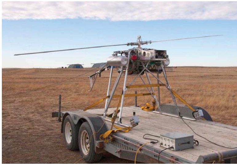
Figure 3 DRDC Suffield's Aphid heavy lift rotorcraft prototype ready for transport (see online version for colours)
