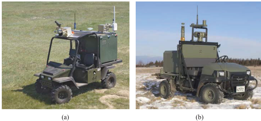
Figure 4 DRDC Suffield’s Ackerman steered unmanned platforms (a) Raptor (b) MATS (see online version for colours)
