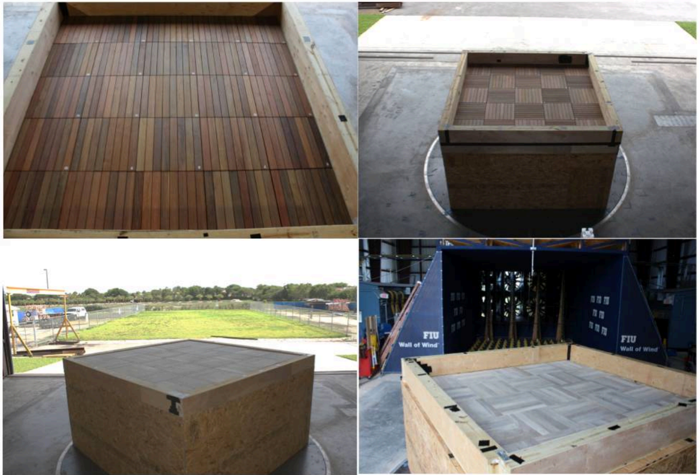
Figure 3 - From top left clockwise: Wood pavers in parallel slats and 12 in. parapet, wood pavers laid out in basket weave and 12. in parapet, porcelain paver with 12 in. parapet and porcelain pavers with 0 in. parapet
