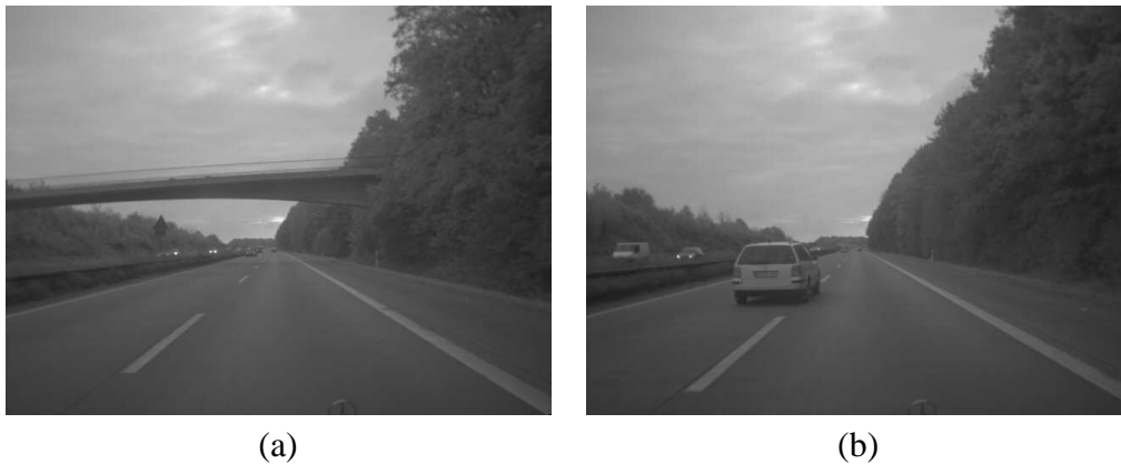
Figure 4.10: The sequence used to investigate the estimation of the pitch angle. A highway was chosen which has a constant vertical slope. The installation pitch angle was obtained by calibration which was \alpha_0 = -4.66^\circ . (a) First frame of the sequence. (b) Frame 100 of the sequence.
