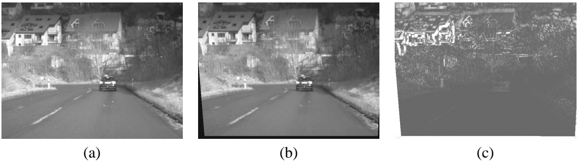
Figure 4.1: Direct method for estimating the ego-motion. The last image (a) is subtracted from the warped current image (b) yielding the difference image (c). The grey-value differences on the road are minimal.
