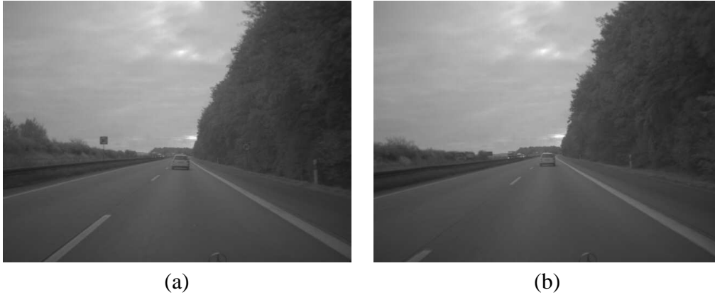
Figure 4.12: Highway sequence with present roll rate. (a) Frame 240 (b) Frame 270. The vehicle has driven approximately 35 meters and it rolled around 3^\circ .
