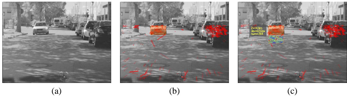
Figure 6.17: Detection of anti-parallel moving objects. (a) An oncoming vehicle. (b) Clustered vehicle. The parallax of the shown correspondences is higher than 2 pixels. (c) The forbidden zone under the vehicle contains a piece of the road. The correspondences are color-coded by their parallaxes. The color goes from blue to red representing a parallax of 0 and 2 pixels, respectively. The zone contains 364 correspondences with a median parallax of 0.52 pixels. The object is revealed as a moving object.
