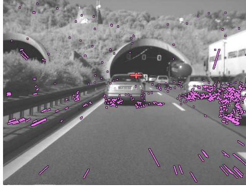
Figure 6.10: Detection of preceding objects. Only the very bottom part of the car in front of the ego-vehicle is detected. The cars on the right hand side are detected to a higher extent.
