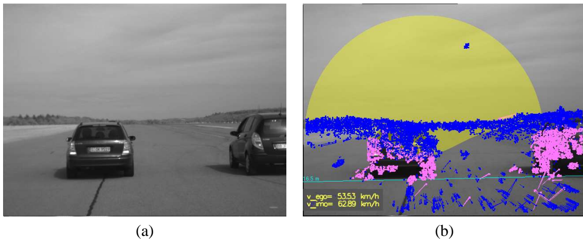
Figure 6.15: Experimental verification. (a) Original image with two moving vehicles in front. (b) The semi-transparent yellow region shows the image region where the motion is not detectable. The measured optical flow vectors are classified as static (blue / dark) and moving (magenta / bright).
