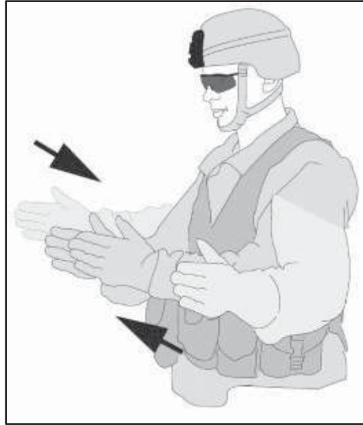
Figure 2-34. Close distance between vehicles and stop
