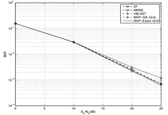
Fig. 2. BER comparison of various detection algorithms for OFDM systems; TU Channel (6 taps), 120 km/h
