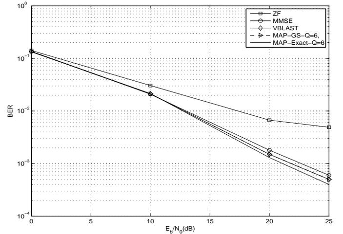
Fig. 3. BER comparison of various detection algorithms for OFDM systems; BU Channel (6 taps), 420 km/h
