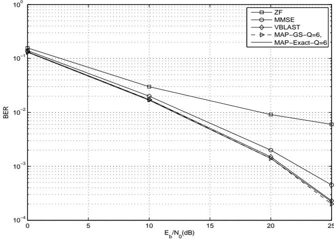
Fig. 1. BER comparison of various detection algorithms for OFDM systems; TU Channel (6 taps), 420 km/h
