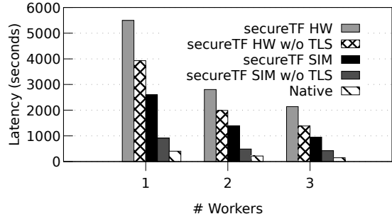
Figure 8. The training latency comparison between SECURETF with different modes and native Tensorflow.
