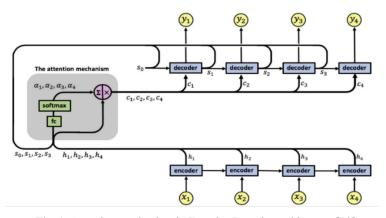
Fig. 1. Attention mechanism in Encoder-Decoder architecture [10]
