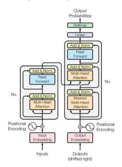
Fig. 2. Transformer Model Architecture [11]
