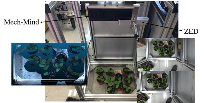
Fig. 3: Data sampling system constructed in this research.
