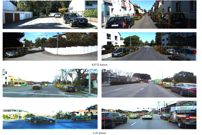
Fig. 4. Visualization of the results on the KITTI and the Lyft validation split sets. The ground-truth 3D boxes and the predicted 3D boxes of our method are drawn in green and red, respectively.
