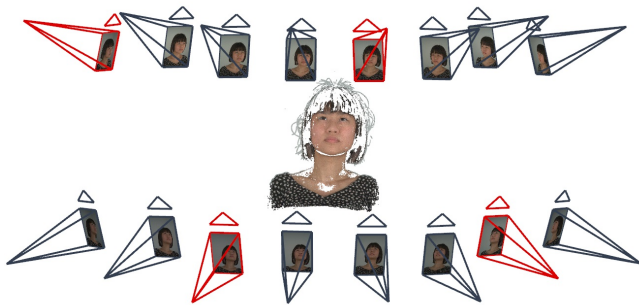
Fig. 7. Spatial layout of our camera setup. Marked in red are the 4 views used for evaluation. The point cloud reconstruction is obtained via COLMAP and used for additional depth supervision.
