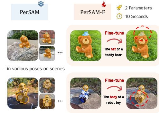
Figure 2: Personalized Segmentation Examples. Our PerSAM (Left) can segment personal objects in any context with favorable performance, and PerSAM-F (right) further alleviates the ambiguity issue by scale-aware fine-tuning.
