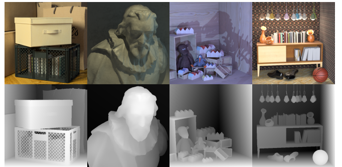
Figure 4: Centre views (above) and respective ground truth disparity maps (below) of light fields from the HCI 4D Lightfield Benchmark. From left to right: Boxes, Cotton, Dino, and Sideboard.
