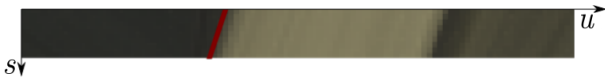
Figure 1: Truncated horizontal EPI from the Cotton light field. The red line indicates the projection of a single 3D-space point.
