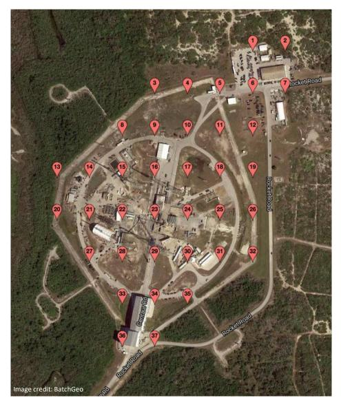
Our analysis of Launch Complex 40 estimates that parts of the launch pad will experience occasional flooding by 2020 and frequent flooding by 2040. For a comprehensive assessment of the launch complex, we mapped a grid of points ~200 ft. apart, allowing us to determine which parts of the launch complex are expected to flood and how often.
