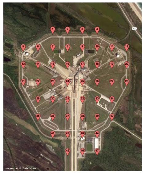
Our analysis of Launch Complex 39B estimates that parts of the launch pad will experience frequent flooding by 2040 and chronic flooding by 2070. For a comprehensive assessment of the launch complex, we mapped a grid of points ~400 ft. apart, allowing us to determine which parts of the launch complex are expected to flood and how often (the spacing of the points for each complex was based on its area).
