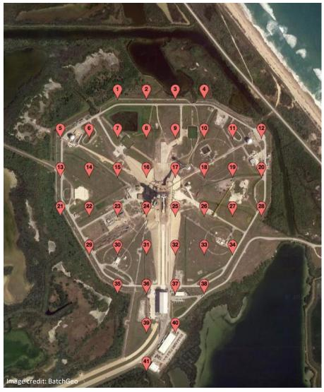
Our analysis of Launch Complex 39A estimates that parts of the launch pad will experience frequent flooding by 2020 and chronic flooding by 2060. For a comprehensive assessment of the launch complex, we mapped a grid of points ~400 ft. apart, allowing us to determine which parts of the launch complex are expected to flood and how often (the spacing of the points for each complex was based on its area).
