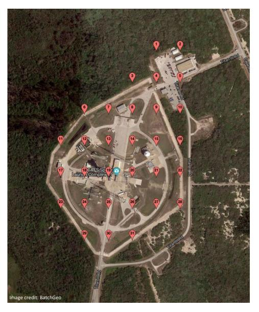
Our analysis of Launch Complex 41 estimates that parts of the launch pad will experience occasional flooding by 2020 and frequent flooding by 2070. For a comprehensive assessment of the launch complex, we mapped a grid of points ~200 ft. apart, allowing us to determine which parts of the launch complex are expected to flood and how often.
