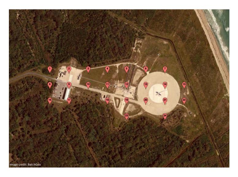
Our analysis of Launch Complex 13 estimates that parts of the launch pad will experience occasional flooding by 2050 and frequent flooding by 2090. For a comprehensive assessment of the launch complex, we mapped a grid of points ~200 ft. apart, allowing us to determine which parts of the launch complex are expected to flood and how often.
