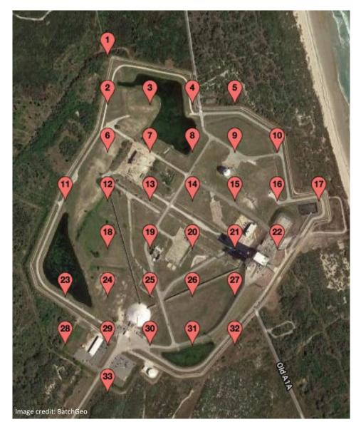
Our analysis of Launch Complex 37 estimates that parts of the launch pad will experience occasional flooding by 2040 and frequent flooding by 2090. For a comprehensive assessment of the launch complex, we mapped a grid of points  $^{\sim}400$  ft. apart, allowing us to determine which parts of the launch complex are expected to flood and how often.
