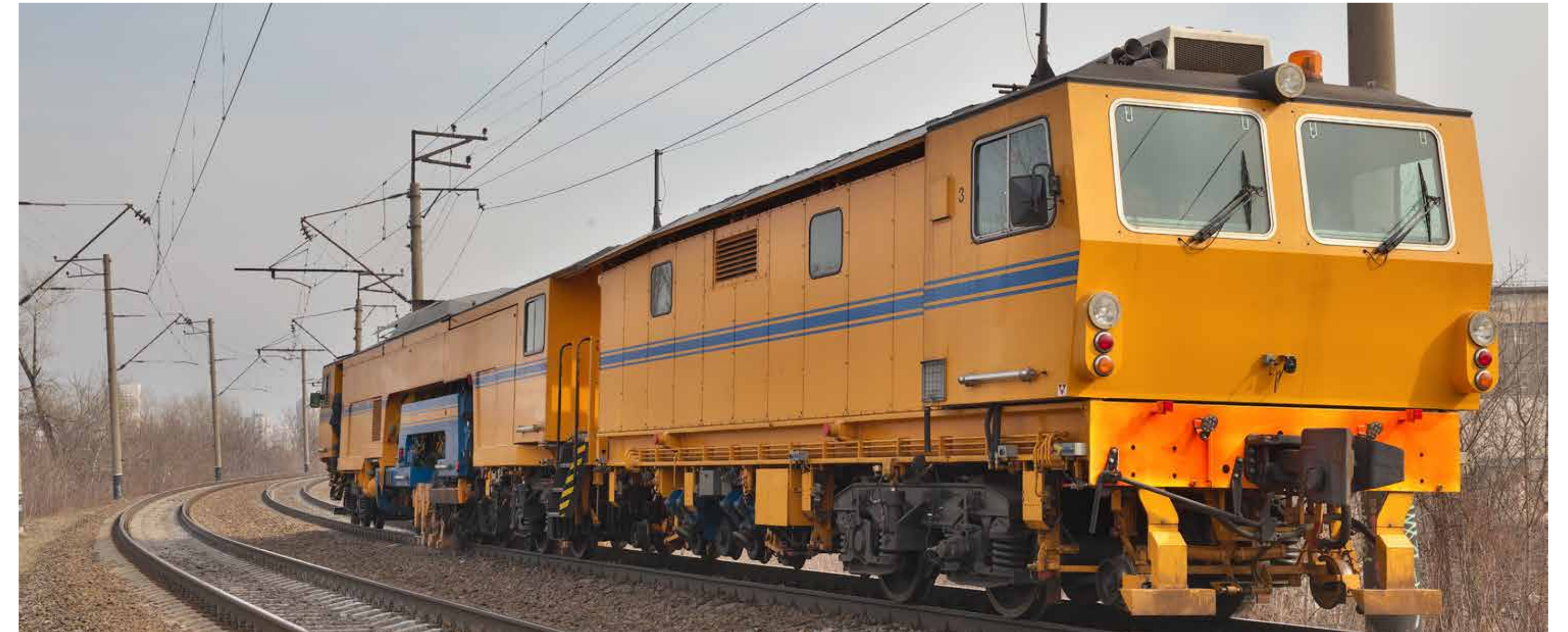
An example of an On-track Maintenance Machine (OTM)
